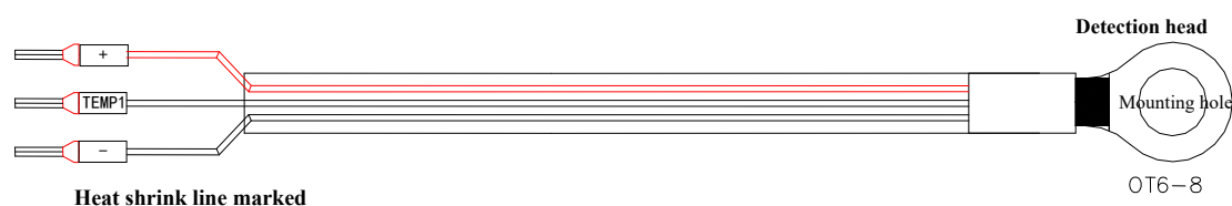
Figure 4. The Shape and Terminal Definition of the Temperature Sensor
